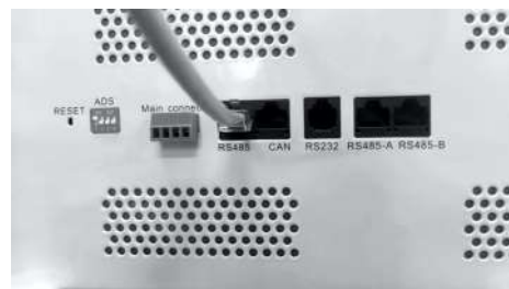
Lithium battery connection diagram
